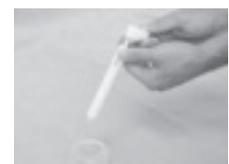
**PRECAUTION:** The magnetic Source Recovery Probe should be held and operated near its release lever in order to avoid unnecessary radiation exposure.
